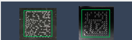
Engraving codes for firing pins on automotive parts
