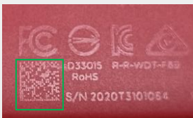
Very low contrast laser engraved code for SSD enclosure
